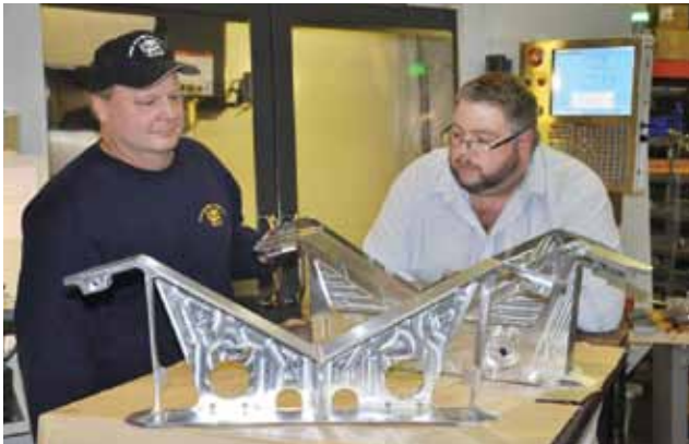
Brian Prigel (left) and production manager John Van-BySteren inspect structural bulkhead components for an unmanned aerial vehicle launcher at Prigel Machine.
